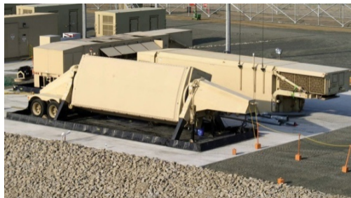
THAAD AN/TPY-2 Radar Electronic Equipment Unit (EEU)
